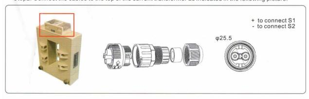
Step3: Connect the other end of the cables to the CT connector provided in the EPM accessory package. S1 connects to + and S2 connects to -.
