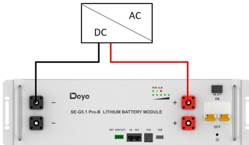
Figure 5-2: Single Battery Connection
