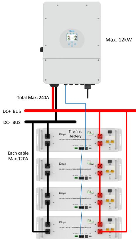
**If the inverter power exceeds 12kW, the parallel mode must be used mode 2!**
