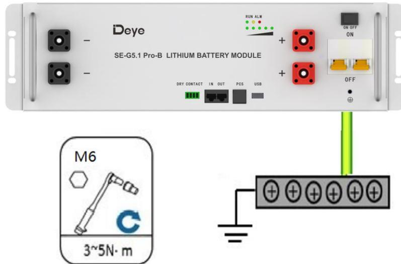
Figure 5-1: Install the Grounding Wire
