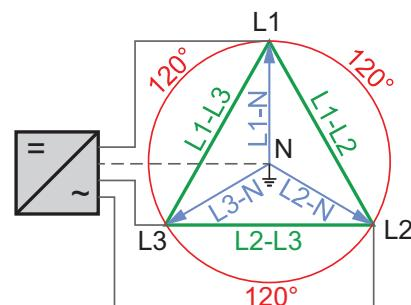
**Hi-Leg Delta** Neutral conductor necessary
