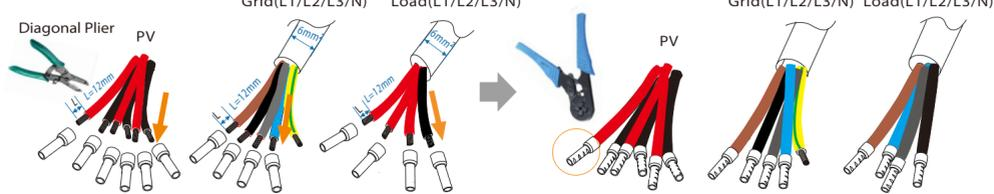
b) Grid(PE) strip the grounding cable insulation (length\*L), insert the stripped cable into the R type terminal, and then clamp it.
