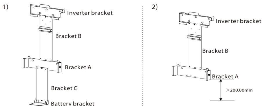
Note: When installing the bracket, be sure to use a spirit level to test and keep the bracket parallel to the horizontal plane. Bracket A should be installed at a distance of 200mm (at least) from the earth.
