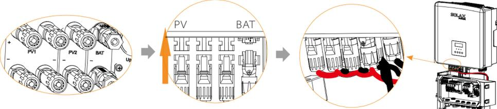
※Note: X3-Hybrid-5.0-M and X3-Hybrid-6.0-M inverters have only two MPPT and two PV strings, so when connecting, you need to unplug ①/② of the PV in the X3-Matebox.
