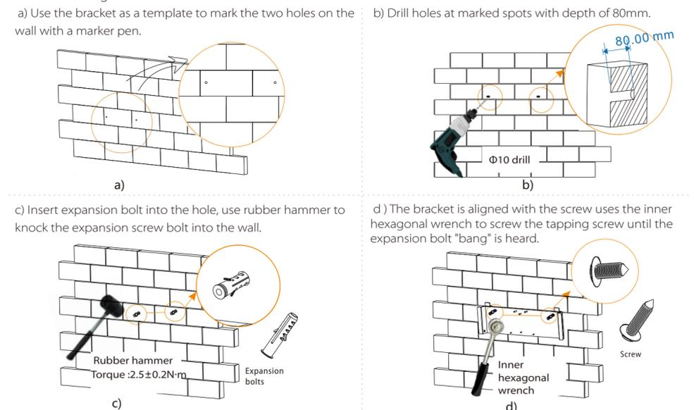
Step 4: Finally, install X3-Hybrid G4 inverter bracket; (Please refer to X3-Hybrid G4 inverter quick installation guide).
