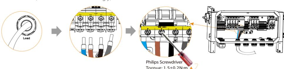
4) Pass the PV /Grid line through the PV port of The X3-MateBox, and then find PV(PV1+/PV1-/PV2+/PV2+) and Grid(R/S/T/N) port inside the X3-Matebox. Force the wire harness directly into the hole to jam, gently twist not to loosen.
