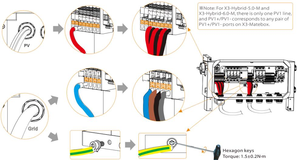
※Note: For X3-Hybrid-5.0-M and X3-Hybrid-6.0-M, there is only one PV1 line, and PV1+/PV1- corresponds to any pair of PV1+/PV1- ports on X3-Matebox.
