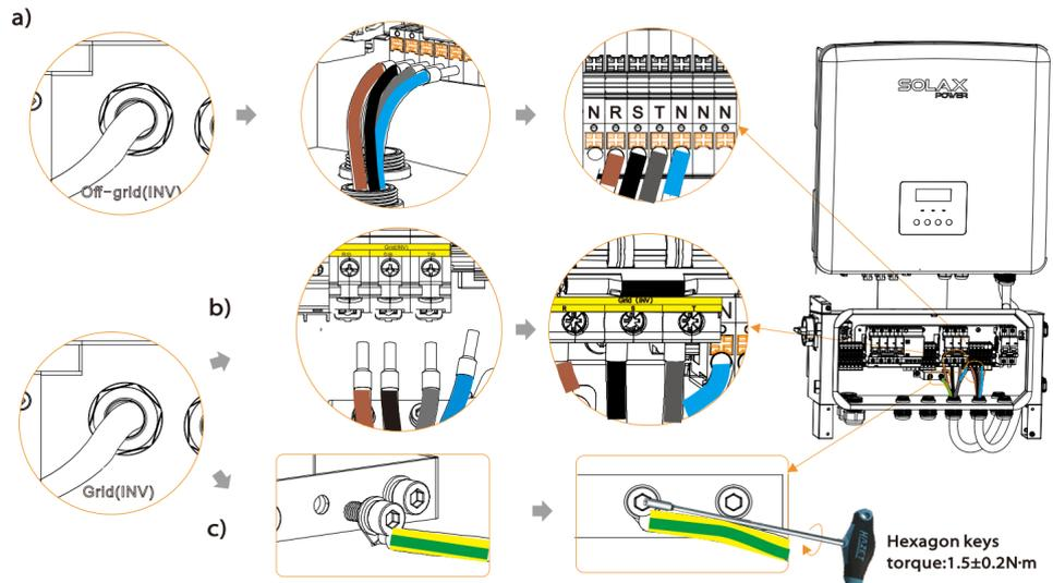
2) PV(PV1+/PV1-/PV2+/PV2-) /Grid(L1/L2/L3/N/PE) /Load(L1/L2/L3/N) side connection
