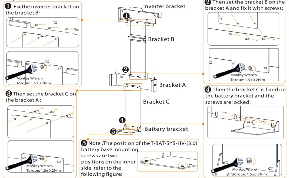
Step 2: Then install the T-BAT-SYS-3.0 battery bracket; (Please refer to T-BAT-SYS-3.0 battery quick installation guide)
