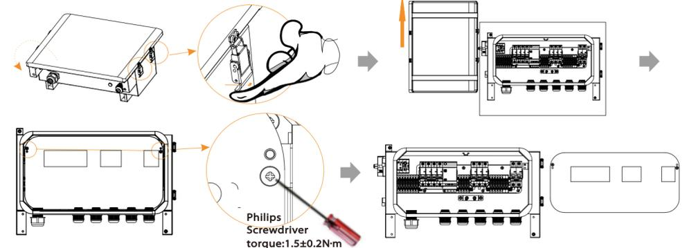
d) Mount X3-Matebox on bracket A and tighten the screws.
