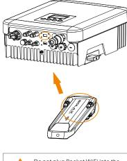
Do not plug Pocket WiFi into the "RF" jack or the "Upgrade" jack. > Tighten the screws with a small Phillips screwdriver
