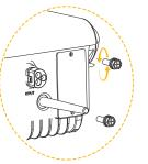
Connect the GPRS module to the DB9 terminal of the PV inverter, and ensure well connecting and no automatic slide.
