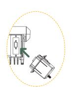
Connect GPRS antenna correctly (before connecting, double check the antenna is of GPRS).
