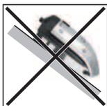
Do not install the inverter on a sloping surface with its connection sockets facing upwards.
